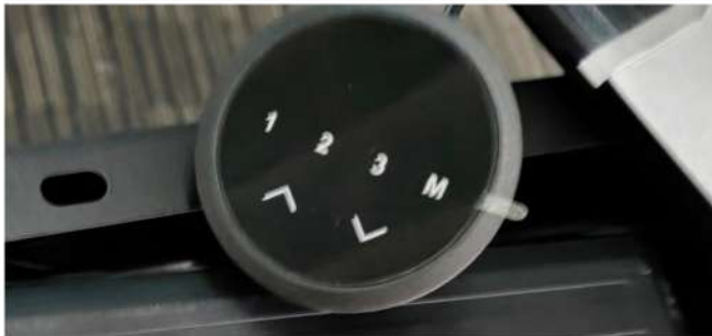
Lift and drop controller
